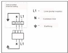
The water pump is supplied by the *L1* and *N* wirings.
